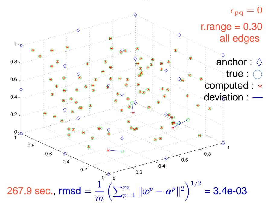
100 sensors, 27 anchors,  $3 \times 3 \times 3$  grid
