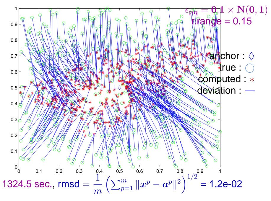
100 sensors and 27 anchors on  $3 \times 3 \times 3$  grid in  $[0, 1]^3$
