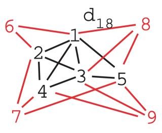
Anchors' positions are fixed. A distance is given for  $\forall$  edge. Compute locations of sensors.
