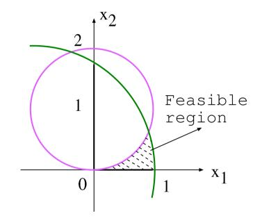
$$egin{aligned} ext{Original problem: max.} & -2x_1+x_2\ & ext{sub.to} & x_1 \geq 0, \ x_2 \geq 0, \ x_1^2+x_2^2-2x_2 \geq 0, \ & \left\|ig( egin{aligned} x_1+1\ & x_2 \end{array} ig)
